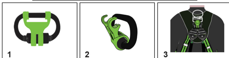
FIGURE 10 - FS1014-TL-BLACK-BWB INSTALLATION
