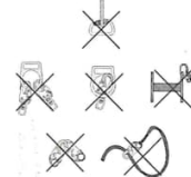
FIGURE 4 - INAPPROPRIATE CONNECTIONS
