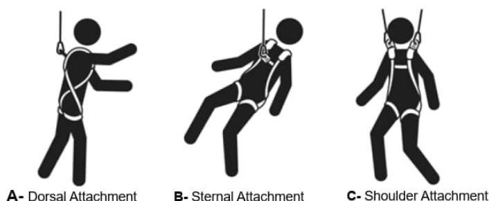
FIGURE 1 - APPROVED D-RING APPLICATIONS
