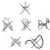
FIGURE 4 - INAPPROPRIATE CONNECTIONS
