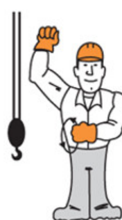
Crawler Crane Travel One Track
