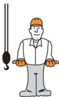
Extend Telescoping Boom
