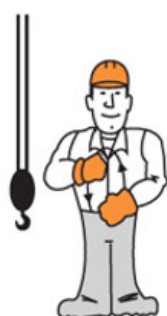
Crawler Crane Travel Both Tracks
