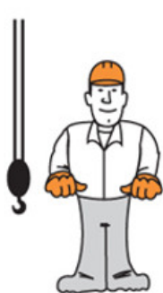
Retract Telescoping Boom
