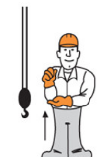
Use Auxiliary Hoist
