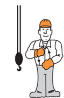
Crawler Crane Travel Both Tracks
