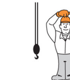
Use Main Hoist
