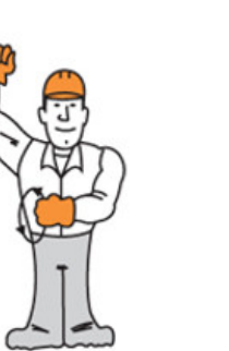
Crawler Crane Travel One Track
