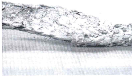
Severe case of compression and construction distortion. Typically this occurs on the bottom layer of a Plasma® winch line compressed against its barrel or flange. If this occurs it is recommended that the severely compressed/ distorted area be cut out before further use.
