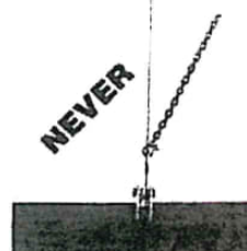
Photograph G. (Typical) Excessive side loading. (J and JA only)
