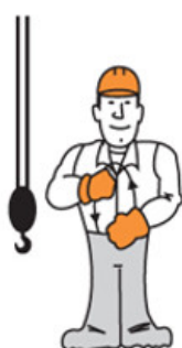
Crawler Crane Travel Both Tracks
