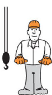
Retract Telescoping Boom
