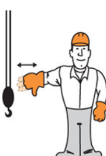
Lower the Boom Raise the Load
