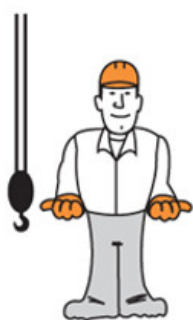
Extend Telescoping Boom
