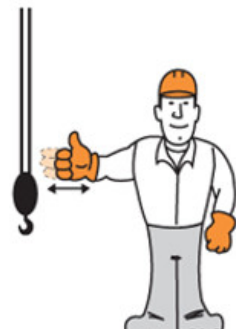
Raise the Boom Lower the Load
