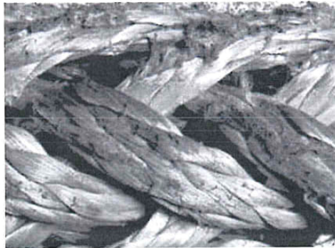
Normal low exterior wear; fuzziness but no cut strands
