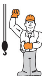
Crawler Crane Travel One Track
